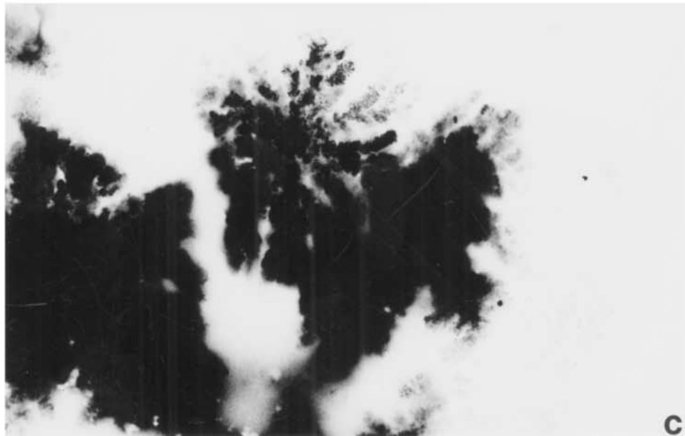
Figure 7 TEM bright-field images of copper deposit structure lifted (extracted) from the surface of aluminum alloy 2524 exposed to basic (pH 11) NaCl solution. (a) Numerous, microdendritic nuclei. (b) Nuclei (arrows) and larger microdendritic clusters. (c) Light exposure view showing microdendritic features in larger cluster marked C in (b).
